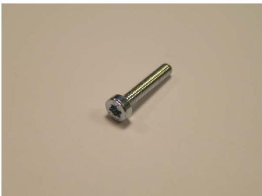
TA013499 TORX-SCREW SN4850 M3x16 TX 8.8 VZ
